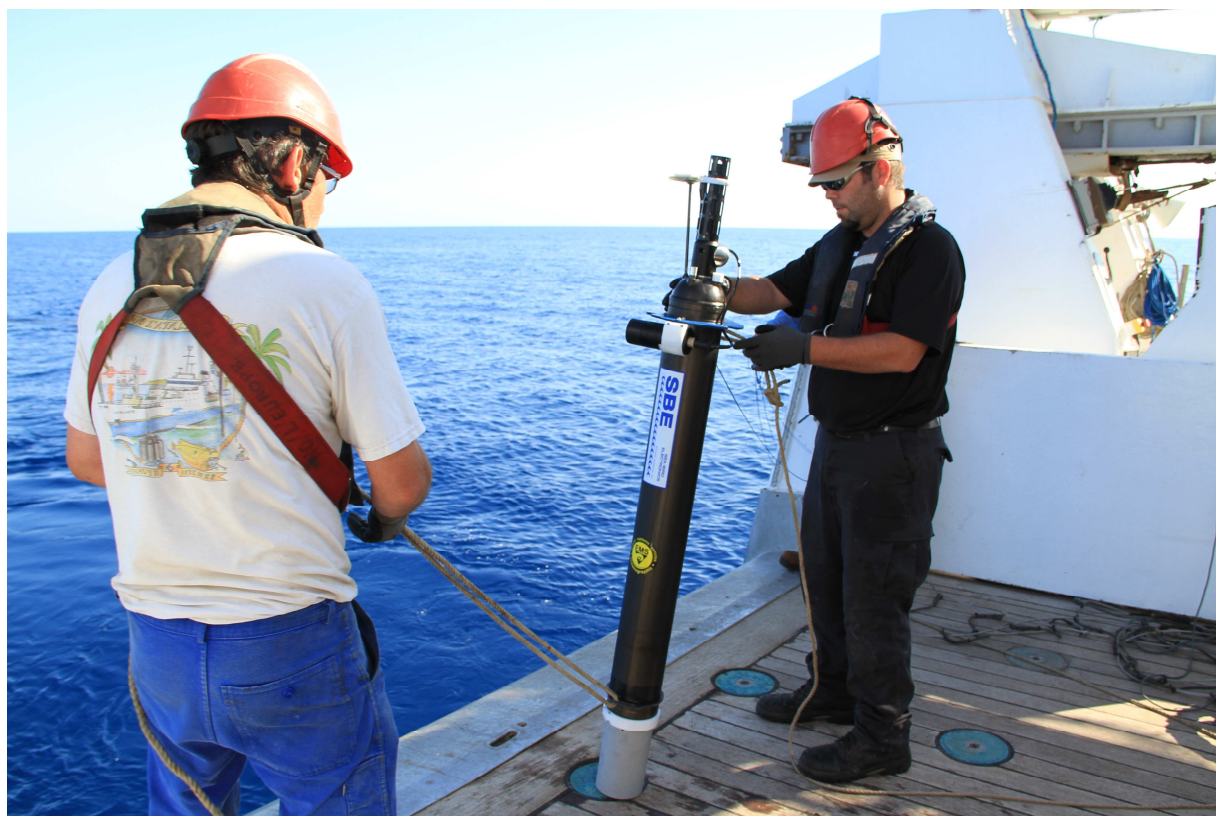
The Sea-Bird Navis autonomous profiling float deployment in the vicinity of the BOUSSOLE buoy.
